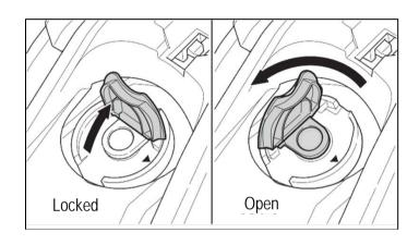
Open the fuel filler cap by lifting upwards, then twist to the left to open the cap.
