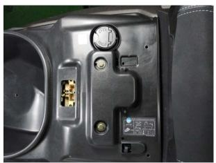
The fuel filler cap can be seen after opening the seat pad.
