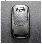
The KEYLESS is the hi-tech electronic main switch that does not need a key (per the figure above). Each vehicle is equipped with 2 sets of remote controllers and they should be preserved carefully. If the wireless key is lost, then you will not be able to open the KEYLESS main switch. For this reason, you are required to preserve the wireless key carefully.
