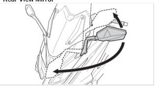
Rear View Mirrors are the important equipment for securing the rider's safety before and during riding. Proper use of the Rear View Mirror is essential. Rear View Mirror is designed to be capable of turning forward and backward. When parking in a narrow space or putting down the vehicle, you may adjust the Rear View Mirror to a proper position.
