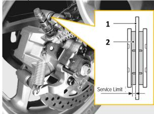
1. Brake Disc 2. Brake Pad Lining
