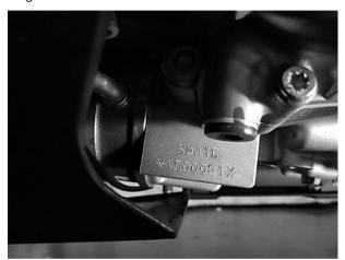
The Engine Number is engraved on the crank box as shown in the figure.
