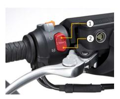
Example : At this position ②, engine is stopped and cannot be started; it requires switching back to "O" position to start the engine.
