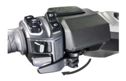
Turn Parking Brake Arm to the left and click into lock position. To unlock, just turn Parking Brake Arm back to its original position (on the right).
