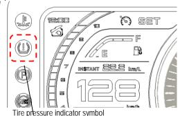
2. When KEYLESS Main Switch is set ON, the Tire Pressure Sensor related Model Symbol on the left side of Dashboard will light up; if this symbol stays on constantly, the tire pressure is not normal (as shown in the Figure).
