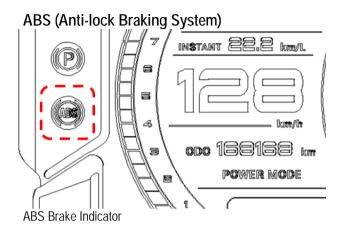
The ABS Brake System is designed in double-electronic control mode. It can be used to activate the front, rear and pedal brakes separately. When ABS is activated, the rider can feel pulses acted by ABS on the handlebar; in which case the rider needs to hold the handlebar constantly, without "press-and-releasing" it, or the ABS effect may be diminished.
