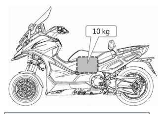
Do Not exceed the following load limits: The maximum load of the storage box shall be limited to 10kg at most. It is forbidden to install a carrying basket or bracket on the front header. Carrying anything in front of the vehicle will surly block the headlight and significantly affect driving safety.
