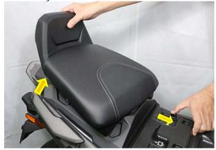
Detach the rear seat pad, and remove the rubber cover of the rear seat pad
