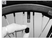
With **Presta valves** you first have to undo the small knurled nut a little and depress it carefully until air starts to escape. Check the nut is tightened and seated in its stem, otherwise air may slowly leak out. Do not forget to tighten the valve by hand nut after inflating.
