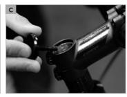
If you want to turn the stem around, you have to also release the bolts of the faceplate securing the handlebars (d). If the stem is fitted with a cap, you can simply take out the handlebars at this point. If it is not fitted with a cap, you have to remove the handlebar fittings.
