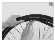
Work the tyre into the rim by approaching the valve symmetrically from both sides. Towards the end, you will have to pull the tyre vigorously downwards (a) to make the already mounted portion of the tyre slip towards the deepest part of the rim well. This will ease the job noticeably on the last centimetres.
