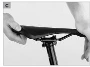
Mount the saddle rails into the inner clamping parts, add the outer parts and re-insert the fixing bolt. If the width of the saddle rails does not fit exactly into the clamp grooves, do not try to force them in. The clamping mechanism or the saddle rails could break and result in an accident and/or injuries to the rider.
