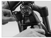
If you have **disc brakes** (hydraulic or mechanic), check the position of the brake pads through the inspection window. In this way you will be able to tell after the removal whether the brake pads are still in their correct position. Read the manual of the brake manufacturer.
