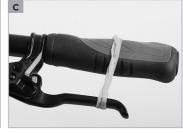
Be sure to transport your SCOTT bike only with the wheels mounted. If transporting your SCOTT bike with the wheels removed, make sure to mount the safety locks. Pull the brake levers and secure them with a strong elastic strap (c) when transporting a SCOTT bike with hydraulic disc brakes (d). This will prevent air from entering the system.
