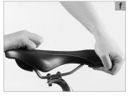
**Clamping with two bolts in line (a)**: Release both bolts two to three turns anticlockwise, otherwise the whole assembly can come apart. Move the saddle forward or backward as desired to adjust the horizontal position. You may have to give the saddle a light blow to make it move. Observe the markings on the saddle rail.
