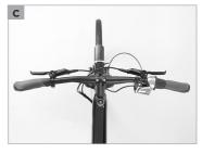
Make sure the stem is firmly fixed by taking the front wheel between your legs and trying to turn the handlebars and stem relative to the wheel **(d)**. If there is movement, you have to increase the torque value. Do not exceed the maximum torque value.
