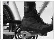
The main advantage is that these clipless pedals (d) prevent your feet from slipping off when pedalling fast. They enable you not only to push but also to pull the pedals. This makes your pedalling more smooth and increases the power transmission compared to normal pedals.
