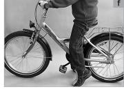
Special attention should be paid to the adjustment of the control elements, such as brake levers. Easy reach and operation should be ensured for the child (a).
