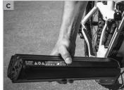
Damage to the outer housing of the rechargeable battery can result in water or moisture entry which can lead to short circuits or electric shocks. The rechargeable battery may catch fire or even explode! In such a case, contact your SCOTT dealer immediately. For more information see the system instructions of your drive manufacturer.
