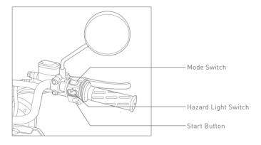
Mode Switch: Press left part to switch to Mode 1[Eco Mode]. Pess right part to switch to Mode 2[Sport Mode].
