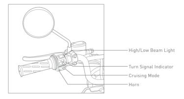
High/Low Beam: Press the right part to turn on the high beam; press the left part to turn on the low beam. To signal overtaking with flashing light, the rider may press and release the Pass button repeatedly.
