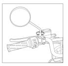
③ Take out the foot rests and assemble the top and holder together with screws for both sides with M6 screws.
